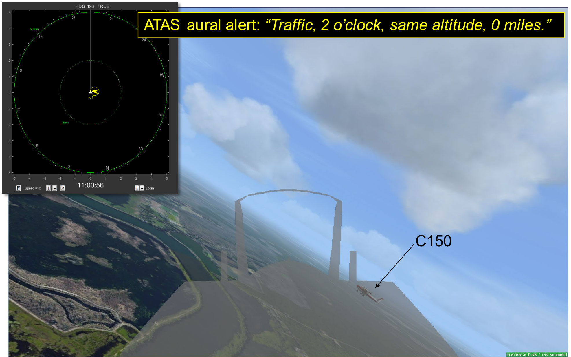
Figure 13. FSX recreation of the view from the F-16 cockpit 0.6 seconds before the collision.
